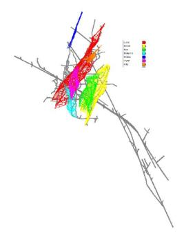
Figure 11: Schematic section showing some of the veins and the extraction adits in the Pimenton mine.
