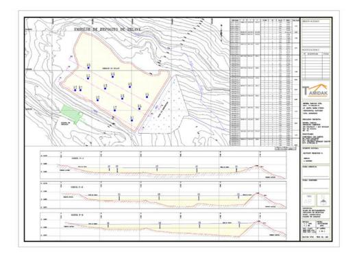
Figure 13: Tailings Pond and sections with the location of the Auger-type holes.
